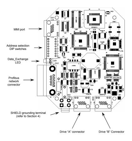
Note that for clarity the above diagram shows the PBDP-110 unit removed from its case. However, it is not necessary to remove the unit from its case in order to install or configure the PBDP-110.
